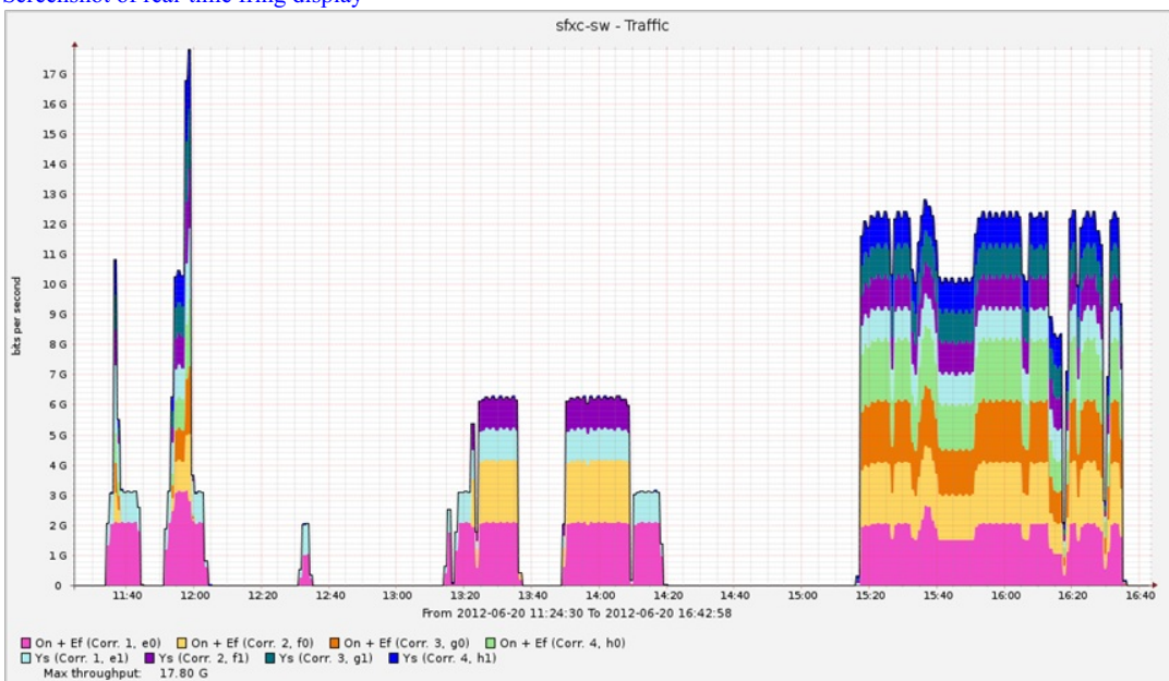
Data throughput at JIVE. The peak of 18Gbps is caused by internal flooding at the correlator
