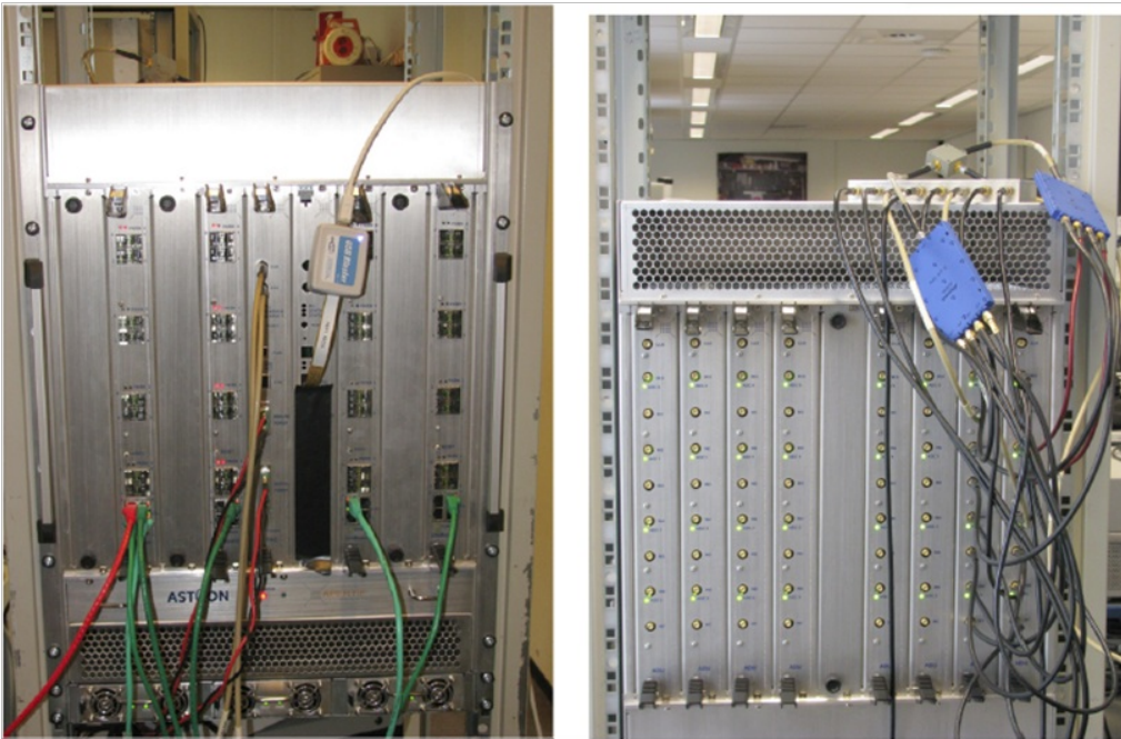
Front and back view of Apertif beamformer sub-rack.
