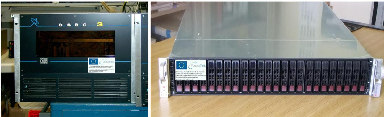
Figure 13: **Left:**The DBBC3L prototype for EVN at 32Gbps **Right:** The FILA40G prototype
