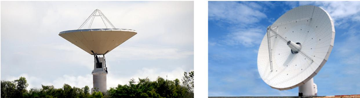
Figure 8: Arecibo 12 m phase-referencing antenna
