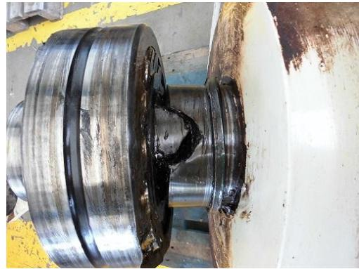
Figure 12: The broken azimuth wheel shaft
