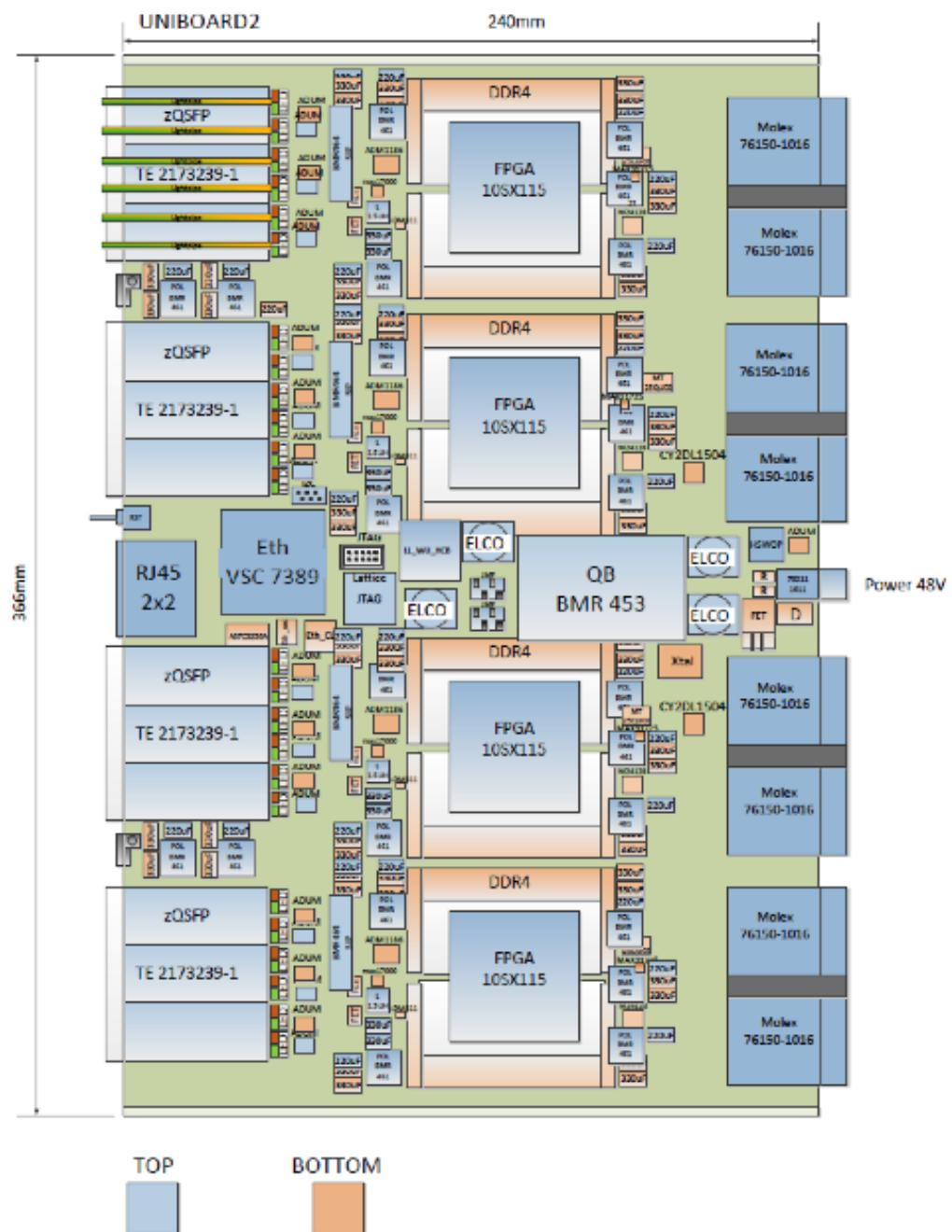
Figure 35: High-level design of UniBoard
