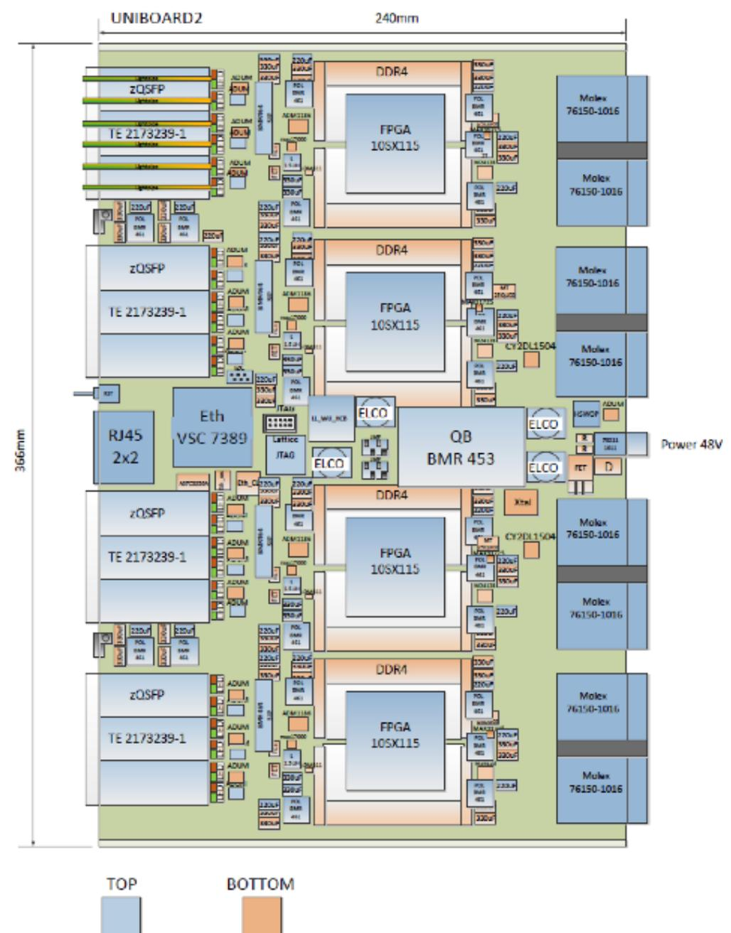
Figure 35: High-level design of UniBoard
