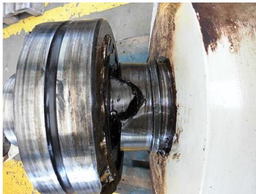
Figure 12: The broken azimuth wheel shaft
